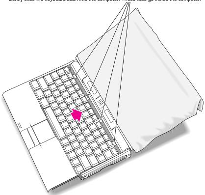
Gently slide the keyboard back into the computer. These tabs go inside the computer.
